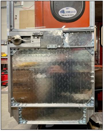
Some of the cars I saw had raised the doorsills, with the bottom of the door straight across.I like the low doorsill of the MT-19, so I made the doors longer with curves around the wheelwells. The door frame corner supports were moved from the doorway to the inside, facing away from the door. The door jams were reinforced with 1 1/2" aluminum angle. A prop-rod was added to keep the door open about 3" for those hot days. They can also be folded all the way back, for that open air feeling.
