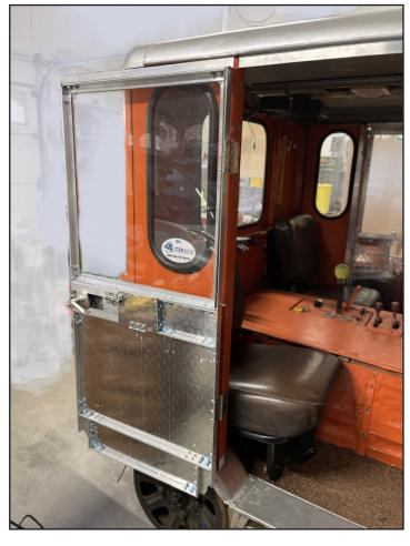
My new doors would be built with 1/8" thick that welding aluminum is much harder than it x 1" aluminum angle for the frame, 1/16" thicklooks. I will never criticize anyone's aluminum aluminum diamond plate panels and a big plexiglass window, all inset in to the "L" brackets.
