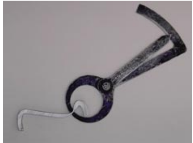
Method of measuring flange/tread interface with wheel thickness gauge.
