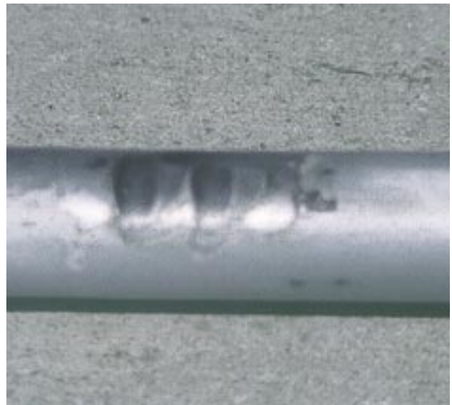
Brake shaft worn nearly half way through. Note twist and bend in shaft from brake application.
