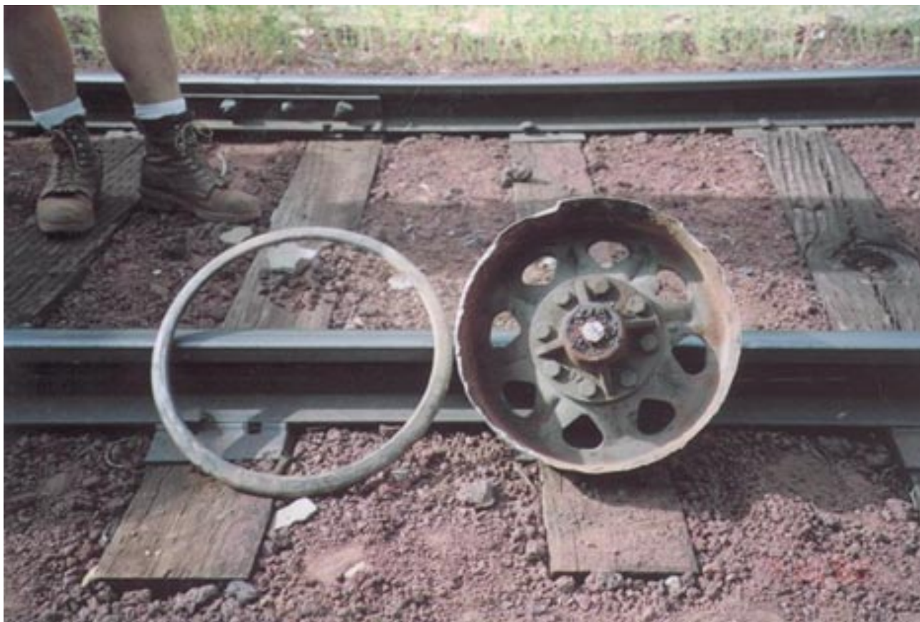
Flange separation from 16" demountable wheel due to flange wear.
