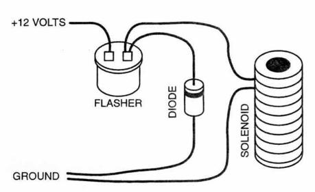
allowing current to pass only one way through it. Any good medium-current diode will do, like a 1N5402 (or better). A Radio Shack 276 1144 will do fine. (They call it an Epoxy Rectifier.) Because diodes are polarity sensitive you'll have to pay attention in hooking it up.
