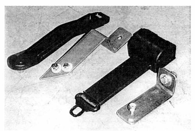
I found a way to make some appropriate brackets to attach the belts to the frame by bending some 3/16" x 2" steel stock. You can see the belts and the the brackets below. On the left is the belt and bracket for the outside of the seat, the right for the inside. The belt on the right has the retractor in it.
