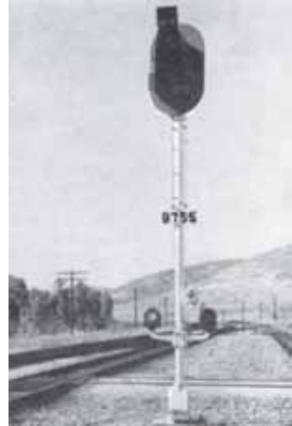
Union Pacific motor car indicators near Echo, Utah; paired sets of three dots mounted low on the regular block signal mast alongside setoff.
